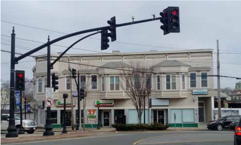
Stoughton, MA: example of parapet roof construction with large cornice and individual roof forms over bay windows with a sign band for first floor commercial uses. The majority of the storefront at the pedestrian level is designed to be transparent.
