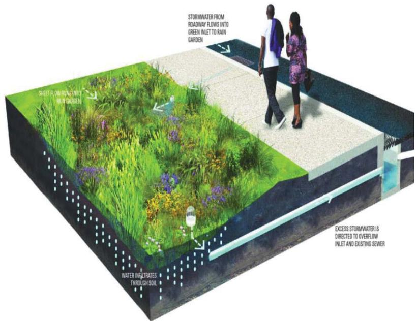
Figure 6-1: Green stormwater infrastructure -rain garden diagram (Source: Philadelphia Water Department)
