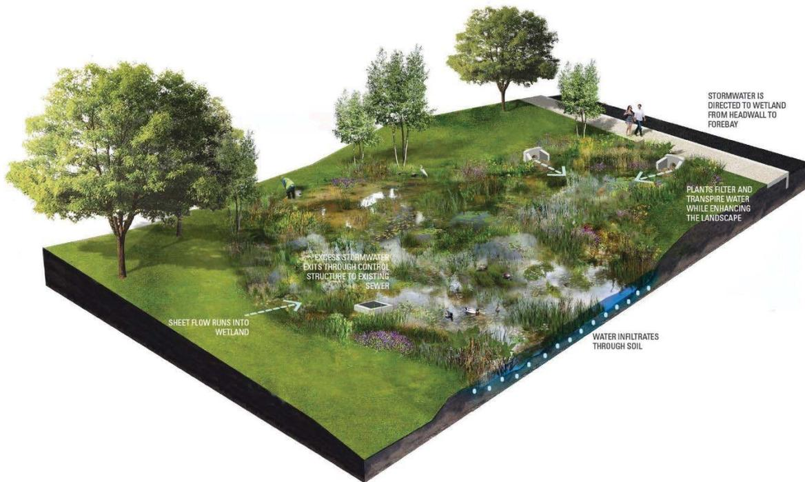
**Figure 6-2:** Conceptual diagram of stormwater wetland (Source: Philadelphia Water Department)
