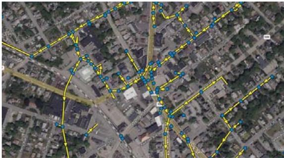
Image of the Town's underground stormwater drainage pipes using the Townwide Model
